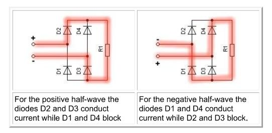
This again results in a DC voltage with ripple. Unlike the case with half-wave rectification the ripple is considerably reduced, and the arithmetic mean and frequency of the ripple voltage have doubled over half-wave rectification.
